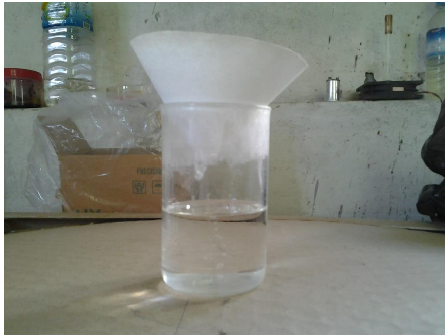
Figure 3.4 The filtered precursor solution for FTO coating.
