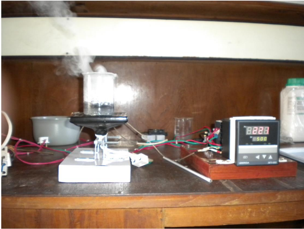
Figure 3.3. The photograph of auto-combustion process (at 500°C).
